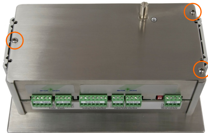
Figure 3-2: Opening the Panel-Mount Enclosure
