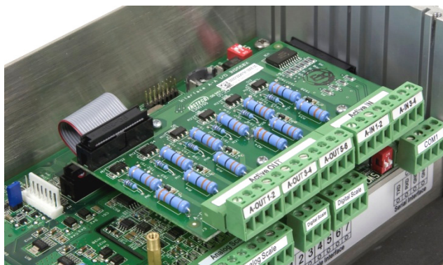
Figure 3-36: Panel-mount Enclosure Discrete I/O Installation
