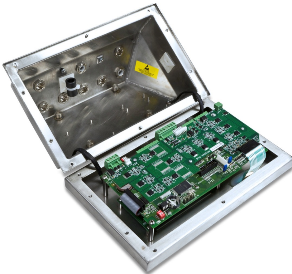
Figure 3-28: PAB Installed on IND560x Main Board
