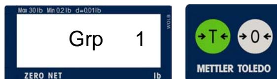
You can press the Tare key to move to Grp 2, 3, or 4. To go into a particular Group, press the Zero Key. Below is what you will see when going into the first Step of Group 1.
