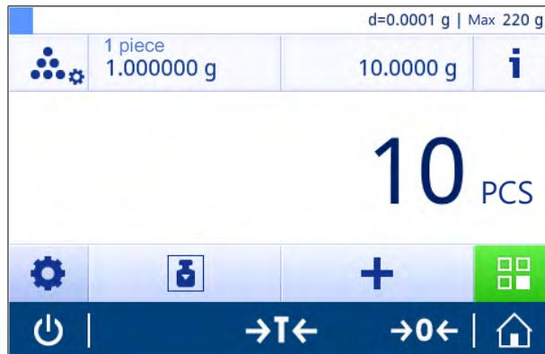
The **Counting** application determines a specific number of pieces based on a predetermined reference piece weight.
