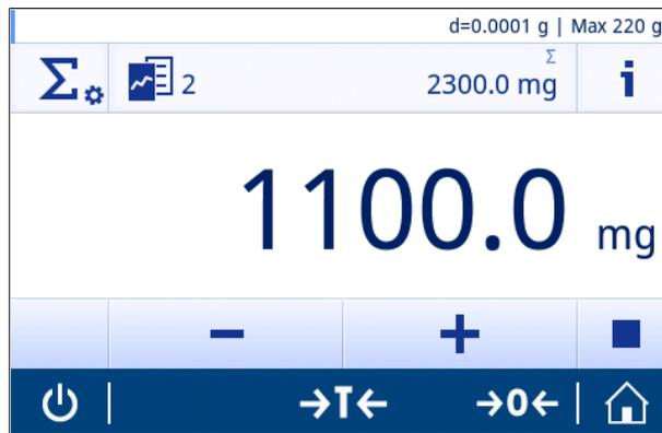
The **Totaling** application allows the user to weigh different samples, add their weight values and totalize them. The application allows the user to:
